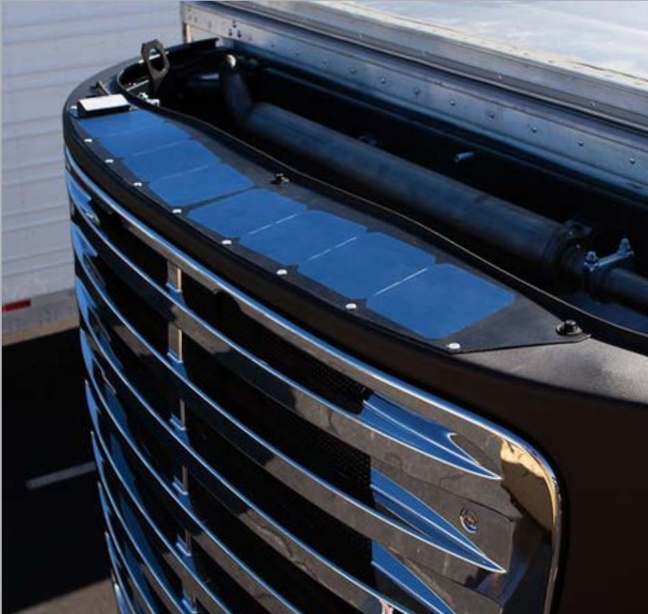
Using high-efficiency SunPower solar cells, we provide cost effective solutions for semi/permanent applications where power density and ruggedness are critical requirements.
